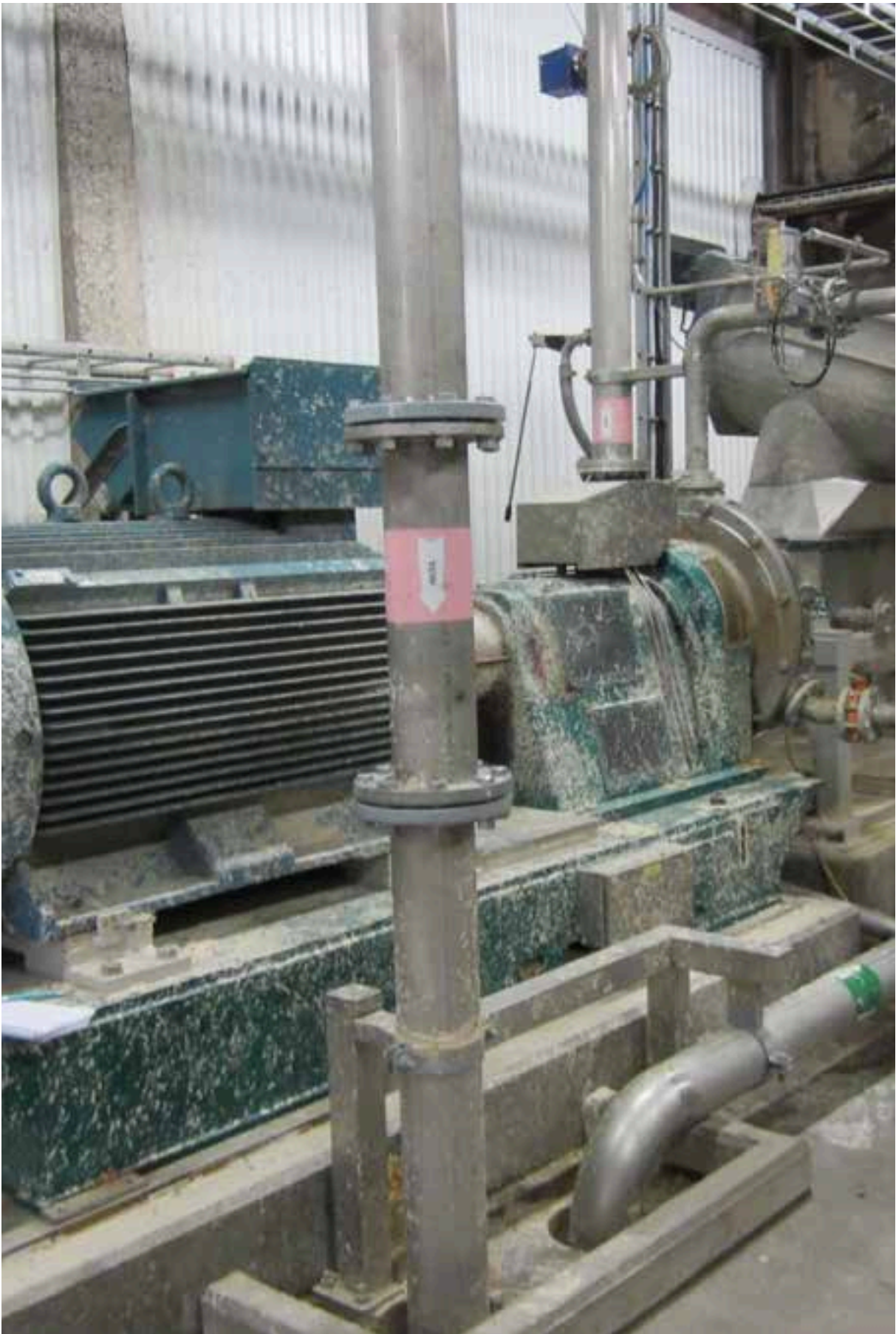
The new Krima disperser is used for treatment of wet-strength broke and storage pulp.
